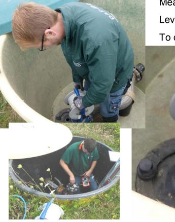
Measurement at gas wells: Level of water & free gas well pipe To drop a perpendicular
