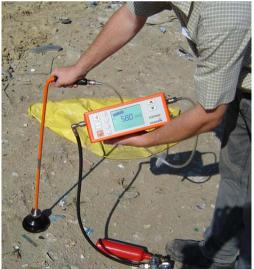
Measurement on surface: (Mesure en surface: ) "VOC" Volatile organic compounds (Les composés organiques volatils)
